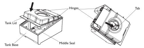
**Note:** If the lid does not close easily onto the base, separate the two parts, reassemble the tank, and inspect it again.
