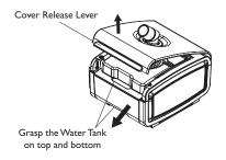
3. Press the tab in the hole on top of the tank in toward the front of the tank. Gently remove the tank lid from the tank base and set aside. Empty any remaining water from the base of the tank.
