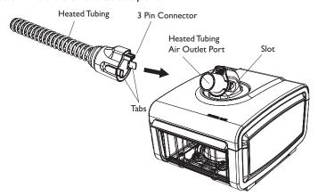
**Note**: Non-heated Philips Respironics tubing (15 or 22 mm) can still be used with this humidifier with the heated tubing air outlet port. Simply connect the tubing to the air outlet port. Refer to the therapy device manual for setup instructions.
