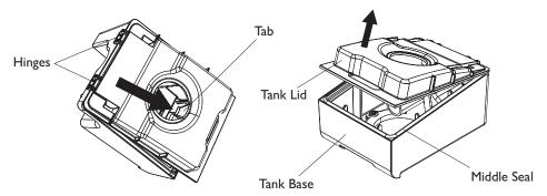
4. Rinse the tank with water. With the water tank sitting on a flat surface, fill it with distilled water (approximately 325 ml) no higher than the maximum fill line located on the front and both sides of the tank.
