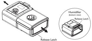
3. If you will be using the therapy device without the humidifier, reattach the side cover to the therapy device.
