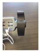
4. Loosen the adjustment knob by turning it toward you.
