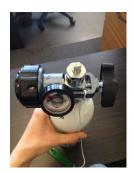
7. Put the regulator over the cylinder post. The pins will slide into the holes.
